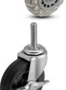
Friction Brake 2", 2-1/2" & 3" models. 2" and 2-1/2" dia. model swivel radius changes to 2-1/8". Add [-B] at end of model.
