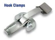
The Bassick Hook Clamp is a general purpose clamp for most common applications. The simple toggle action mechanism combined with a high-tensile alloy steel spring exerts a clamping force of 50-75 lbs when actuated. The clamps operate easily, hold well and are ideal for most simple fastening operations. Several Clamp and Strike styles are available for added variety and versatility. Contact Customer Service for individual clamp and strike specifications.
