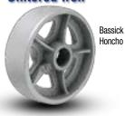
Sintered Iron wheels are powdered iron molded under pressure and sintered providing strong, concentric, smooth faced wheels.
