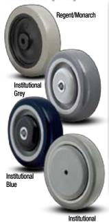
Thermoplastic Urethane Wheels (TPU) consist of a high-grade urethane tread mechanically interlocked to a polyolefin core. The urethane tread offers extended wear, protects floors and resists chemicals and oils.
